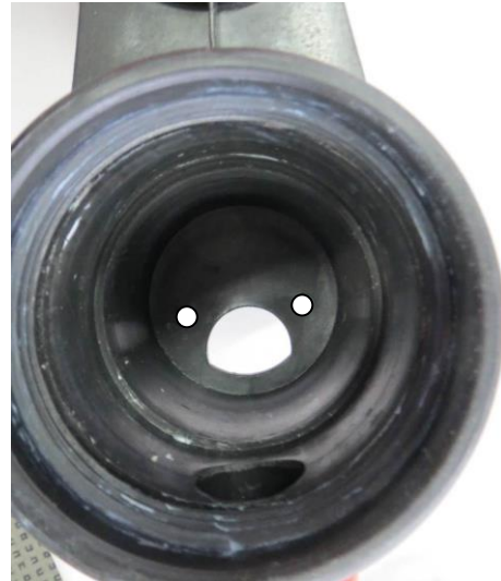
old filter housing with 2 screws
