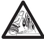
**WARNING!** Kickbacks can be sudden, rapid and violent and can cause life threatening injuries. Read and understand the instructions in the manual before using the machine.
