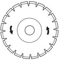
There is an arrow on the machine that indicates the axle's direction of rotation that the disc is mounted on.
