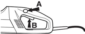
The power switch lock remains depressed as long as the power switch is depressed. When the grip on the handle is released both the power switch and power switch lock are reset. This movement is controlled by two independent return springs. This position results in the machine stopping and the power switch being locked.
