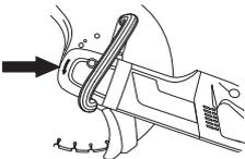
When the blade is replaced with a new one, check the flange washers and the drive axle. See instructions under the heading Checking the drive axle and flange washers.
