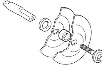
Do not use warped, notched, indented or dirty flange washers. Do not use different dimensions of flange washers.
