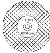
Ensure the blade it not cracked or damaged in any other way.
