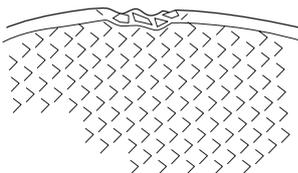
Test the abrasive disc by hanging it on your finger and tapping it lightly with a screwdriver or the like. If the disc does not produce a resonant, ringing sound it is damaged.
