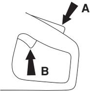
The switch lock remains pressed as long as the switch is pressed. When you release your grip on the handle this resets both the switch and the switch lock. This takes place via two independent return spring systems. This position causes the machine to stop and the switch to be locked.
