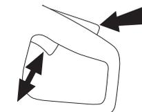
Start the machine, release the switch, and check that the machine and blade stop.
