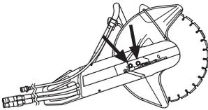
Screw the adjuster screw so that the square headed nut comes opposite the marking on the cover. This automatically ensures that the belt has the correct tension.
