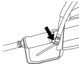
Check that the switch and switch lock move freely and that their return spring systems function.
