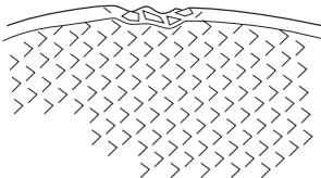
Test the abrasive disc by hanging it on your finger and tapping it lightly with a screwdriver or the like. If the disc does not produce a resonant, ringing sound it is damaged.
