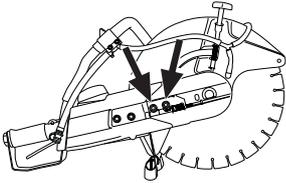
Screw the adjuster screw so that the square headed nut comes opposite the marking on the cover. This automatically ensures that the belt has the correct tension.
