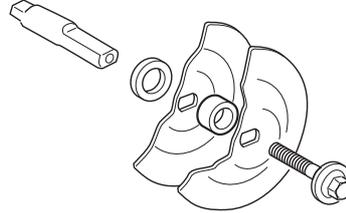
Do not use warped, notched, indented or dirty flange washers. Do not use different dimensions of flange washers.
