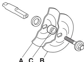
Tightening torque for the bolt holding the blade is: 15-25 Nm (130-215 in.lb).
