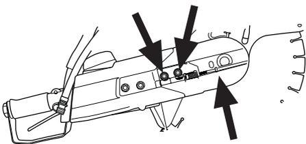
Unscrew the nuts and lift off the front belt guard.
