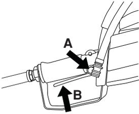
The switch lock remains pressed as long as the switch is pressed.
