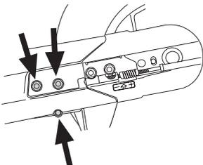
Take off the old belt and fit the new one. Fit the cutting arm to the machine and tension the belt with the adjuster screw. A new drive belt should be re-tensioned after running for about 30 minutes.
