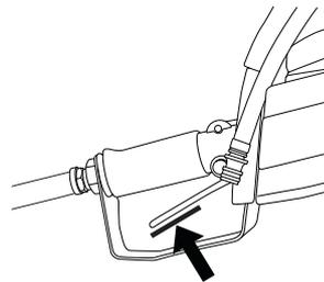
Press the switch lock and check that it returns to its home position when released.
