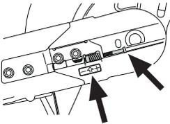
Tighten the two nuts holding the cutting arm.
