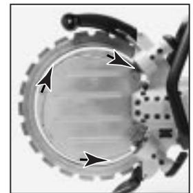
In addition to leading water to the cutting edge, the water disc also supports the blade to prevent twisting and thus helps ensure a straight cut.
