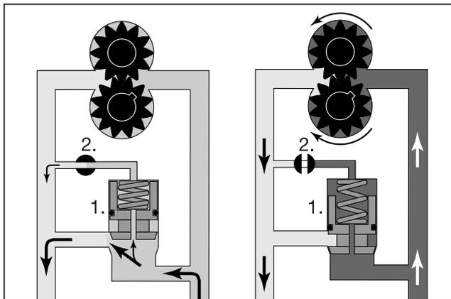
In order to understand the operating principle, we must first examine a few vital components. The main valve (1) has a very small opening that permits a small volume of fluid to flow through the piston, after which it passes the servo valve (2) when this is open. The servo valve is operated on mechanically by the throttle action. A weak spring, which tends to pull the main valve downwards, is also featured. This spring is needed to be able to switch between start and stop.
