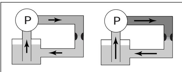
In the diagram on the left, the flow rate is slow and the pressure difference on the two sides of the restriction is very small.
