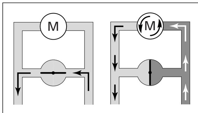
By leading some of the fluid directly to the return side, the flow to the tool can be varied. This principle is used for throttle control in Partner hydraulic cutters. When the machine is not operating, the entire flow passes virtually without pressure through the bypass valve. When the throttle control is pressed in, the bypass valve is closed and the hydraulic fluid is forced to pass through the motor.
