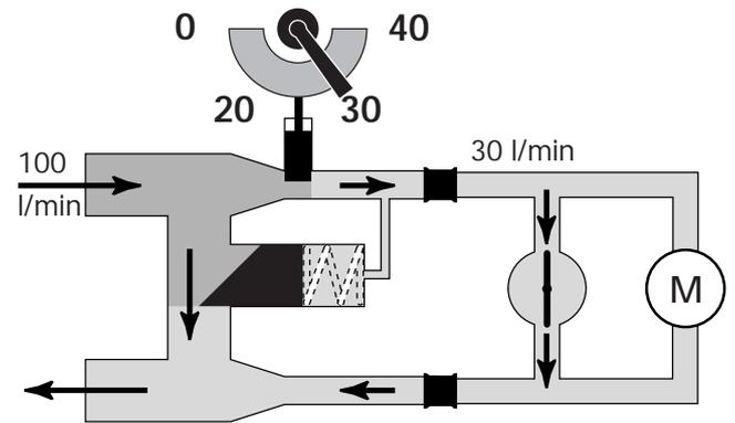
In the above figure, the flow-rate selector is set at 30 l/min. The inlet to the FC40 is partially restricted and most of the fluid passes through the flow valve directly to the return side.
