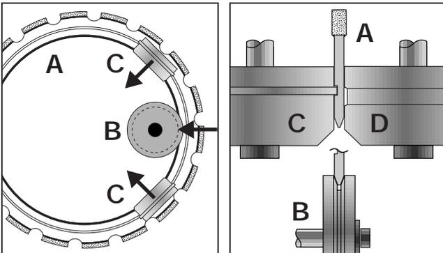
The unique concept behind the K3600 is the eccentric drive of the cutter blade. If the drive system had not given the machine such unique properties, then it would scarcely have made it to the market today. Eccentric drive in practical implementation has imposed considerable demands on development resources and is continuing to place major demands on day-to-day production.
