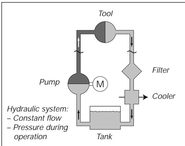
As we said earlier, a fluid cannot be compressed, which means that as long as the pump runs at a constant speed, the flow in the system is also constant, which is exactly the opposite of the compressed-air system.
