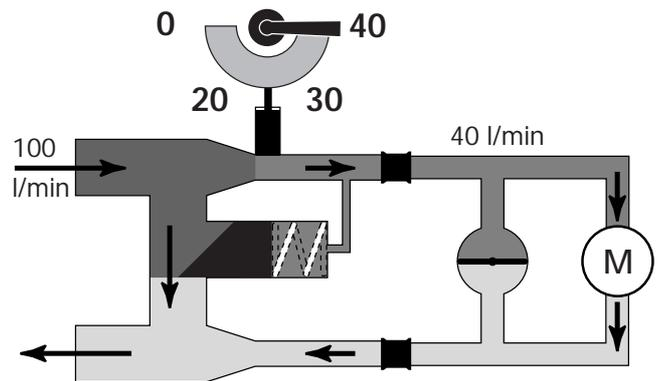
A Partner cutter is put to work (40 l/min). The pressure (resistance) increases in the supply line. This pressure is also led through the narrow duct to the rear of the flow valve, pushing it to the restricted setting. The higher the pressure in the feed line, the firmer the restriction and vice versa. Flow to the tool remains constant.
