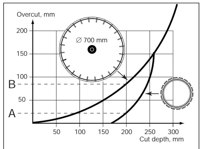
Wall thickness in the above examples is 200 mm. The two upper figures show overcut with the Partner K3600 and a centre-driven cutter (diameter 700 mm). The third figure shows the corresponding cuts as viewed by the operator and in cross-section. The diagram shows the need for overcutting with the K3600 and a centre-driven cutter respectively, at various cutting depths.
