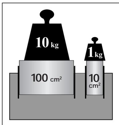
pistons, one with an area of 100 cm<sup>2</sup> and the other just 10 cm<sup>2</sup>. We place a weight of 1 kg on the smaller piston and 10 kg on the large piston. The following will apply:
