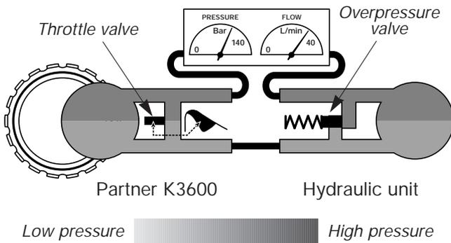
The pressure side of the hydraulic system is described by the upper half and the return by the lower half. As we shall see, there will be no change of pressure on the return side, only the flow path is changed under certain circumstances. That is why we only need to measure what happens on the pressure side, that is to say the side to which the hydraulic unit provides flow and pressure, and which drives the power cutter.
