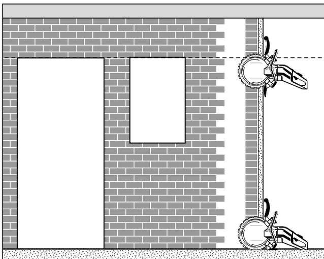
which will be entirely covered by the frame around the door or window. If the cut is made from two directions at the end points, overcut can be eliminated completely at cutting depths of up to 340 mm!
