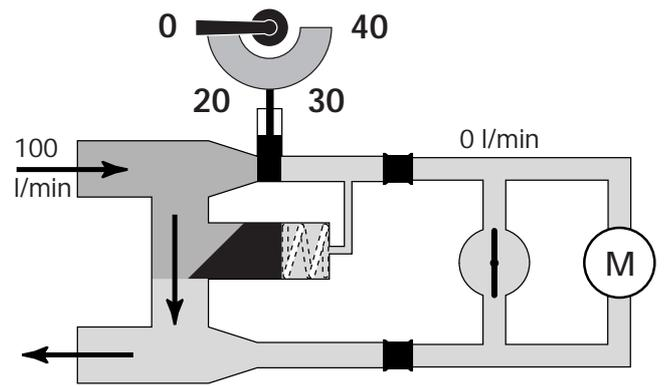
We can first study the function of the flow-rate selector. This is set at "0", the duct is closed and the full volume of fluid must be fed back to the return side. Flow from the pump presses the spring-loaded flow valve to the side and allows the fluid to pass under relatively low pressure.
