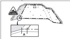
For slopes adjacent to a public road, put a barrier of minimum 15 cm / 6 in. along the outer edge of the slope. You can use a wall or a fence as a barrier.
