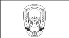
Release the latch of the connector (A) and pull it upwards.
