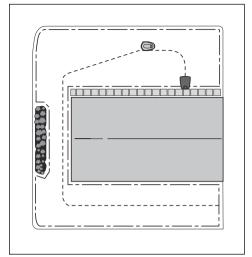
If it is necessary, you can install the guide wire in a loop. Put the guide wire in a loop to the right from the charging station. Put the guide wire at a minimum distance of 1.5 m / 4.9 in. (A) from the other section of the guide wire.
