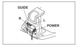
Switch the connections between the guide wire and the boundary wire in the charging station.
