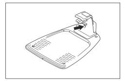
Check that the boundary wire connections to the charging station are properly connected and not damaged. Check that the indicator lamp in the charging station is still flashing blue.
