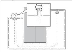
a) Put the 2 ends of the boundary wire and the end of the guide wire into the coupler.
