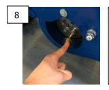
When the drive-motor and wheel are aligned, the quick release pin will lock into place. Close wheel guard.
