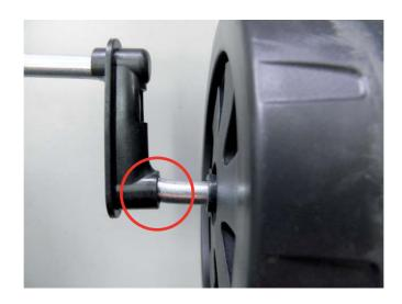
**Field fix:** For products already on market a fix were a washer and new starlock washer is added helps the problem. A permanent fix will be implemented in production as soon as possible.
