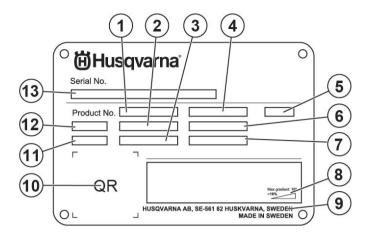
Figure 1-1. Machine name plate
