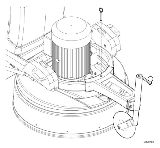
Figure 4-5. Fitting the support wheel
