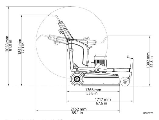
Figure 8-2. Height and length of the machine
