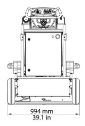
Figure 8-1. Width of the machine
