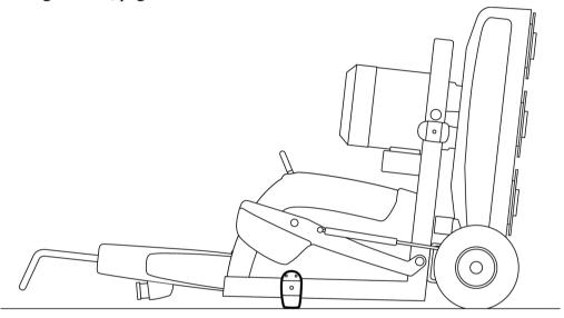
Figure 4-11. Weight lock on the floor
