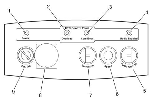
Figure 3-3. Description of controls - Control panel
