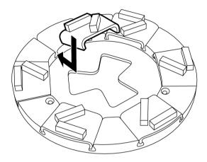
Figure 4-13. Fitting grinding tools
