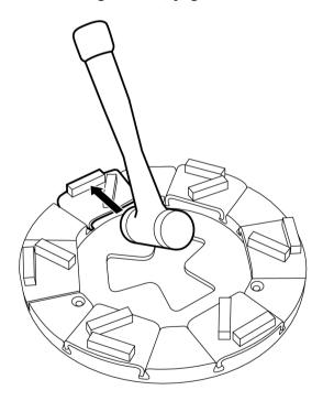
Figure 4-14. Removing grinding tools
