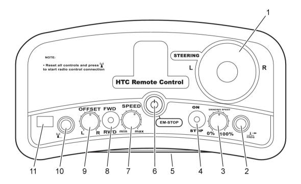
Figure 3-4. The radio control unit
