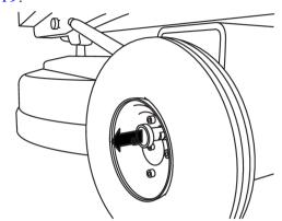
Figure 4-3. Decouple the wheels
