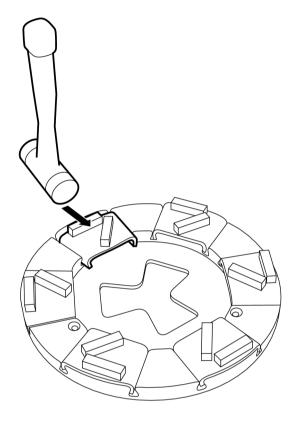
Figure 4-15. Removing grinding tools
