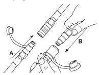
**CAUTION!** Two hose kits can be connected when hose lengths exceeding 18 m are required. Do not connect more than two kits as the couplings cause large power loss. See the Technical data.
