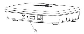
The smart Gateway will be reset to the factory settings. You may need to use the reset function if for example you want to link your Gateway to a new Wi-Fi network.
