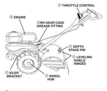
①SAE 30 OR 10W-30 MOTOR OIL ②REFER TO MAINTENANCE "ENGINE" SECTION ③EP #1 GREASE
