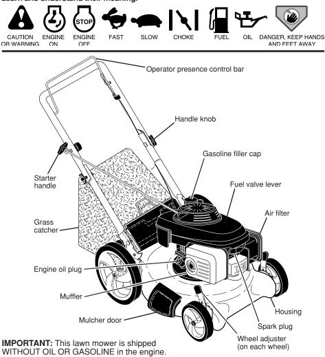
NOTE: Gasoline containing up to 10% ethanol (E10) is acceptable for use in this machine. The use of any gasoline exceeding 10% ethanol (E10) will void the product warranty.
