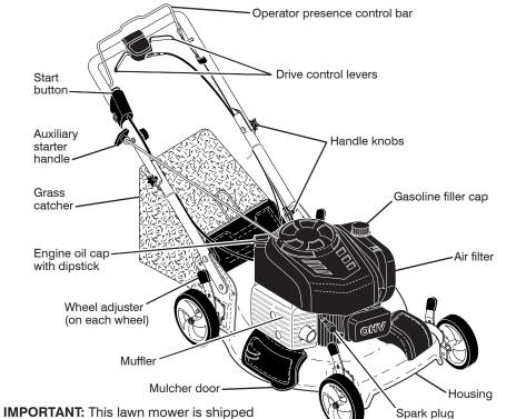
WITHOUT OIL OR GASOLINE in the engine. NOTE: Gasoline containing up to 10% ethanol (E10) is acceptable for use in this machine. The use of any gasoline exceeding 10% ethanol (E10) will void the product warranty.
