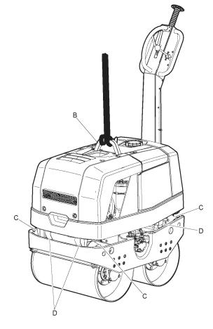
Make sure that the shock absorbers (C), safety straps (D) and the hook (B) are correctly attached and not damaged.
