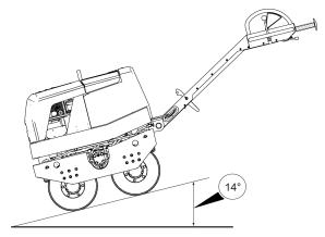
The maximum gradeability of the machine with vibration switched off is 19°.
