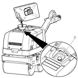
4. Fill the sprinkler water tank (D) with water.
