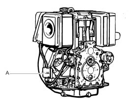
3. When fitting the new filter make sure that the arrow on the filter coincides with the direction of flow of the fuel.
