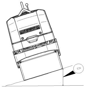
The tilting angle is measured on a hard level surface with the machine stationary. Vibration switched OFF and all tanks full.
