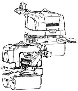
Check the screws on the safety straps, if necessary tighten or replace.
