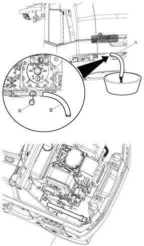
2. Remove the drain hose and screw the drain valve cover (A) back on and make sure there is no leakage.
