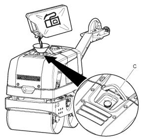
4. Never overfill the tank. Due to the movement of the fuel within the tank, it is possible to have fuel at a higher level than the tank cap, which can lead to a spillage of fuel if the tank cap is opened. This can be avoided by only opening the tank cap when the machine is on level ground and the tank cap is at the fuel tank's highest point.
