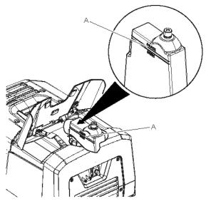
• Fill up with hydraulic oil if necessary, see "Hydraulic system, changing the oil".
