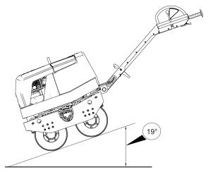
The inclination angle is measured on a hard level surface with the machine stationary. Vibration switched OFF and all tanks full.
