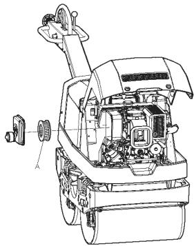
If the filter is contaminated by dry dust, tap the filter against the palm of the hand until all loose dust is dislodged.
