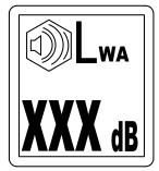
The label indicates the guaranteed noise level corresponding to EC-directive 2000/14/EC. See "Technical data" for accurate noise level.
