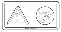
Instruction manual. The operator must read the safety, operation and maintenance instructions before operating the machine.
