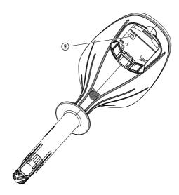
→ Push the Reset key ⑨ for a short time. New connection.
