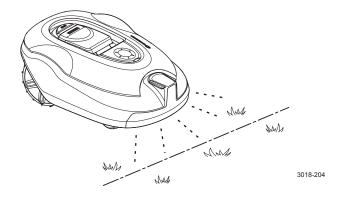
The **STOP** button on the top of the robotic lawnmower is mainly used to stop the robotic lawnmower when it's running. When the **STOP** button is pressed a hatch opens, behind which there is a control panel. The **STOP** button remains pressed in until the hatch is closed again. This together with the **START** button acts as a start inhibitor.
