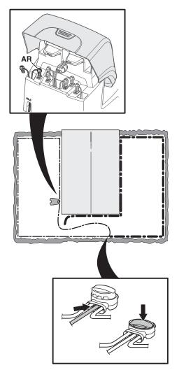
In that case, move the connection for the new wire closer to the disconnected end (roughly at the middle of the suspected wire section) and check again if the indicator lamp is green.
