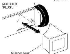
MULCHER PLUG BUILT INTO REAR DOOR
