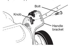
Raise lower handle section to operating position and squeeze the bottom ends of lower handle towards each other until the pin in handle can be inserted into one of the three height adjustment holes.
