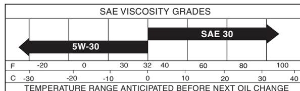
**CAUTION!** Although multi-viscosity oils (5W30, 10W30 etc.) improve starting in cold weather, these multi-viscosity oils will result in increased oil consumption when used above 32°F. Check your engine oil level more frequently to avoid possible engine damage from running low on oil.
