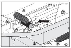
Engage the park brake, pulling the lever upwards.
