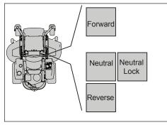
For example, to turn right while moving forward, move the right control towards the neutral position. The rotation of the right wheel is reduced and the machine turns to the right.
