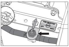
The fuel shut off valve is located at the right rear of the seat. The valve has three positions: right tank, left tank and OFF.
