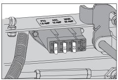
Fuses are located on the right hand side of the machine and are accessed by tilting the seat forward. Fuses are flat pin fuses type as used in automobiles. The 20 A is the primary fuse. The 7.5 A is for the mower deck coupling. The 10 A is for accessories.
