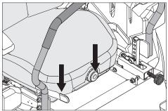
The seat can be adjusted lengthways with the lever located at the right side of the seat (as seen by the driver in the seat). When making adjustments the lever is moved upward.
