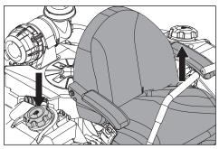
Read the safety instructions before refueling. The capacity for each tank is 5-1/2 gallons.
