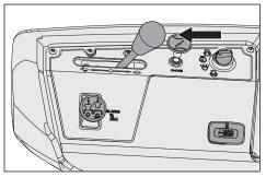
The throttle control regulates the engine speed and the rate of rotation of the blades, assuming the blade switch is pulled out.
