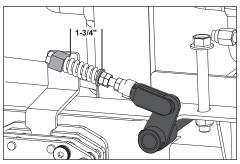
If adjustments are needed, loosen B jam nut and turn A jam nut until the correct distance is achieved. Retighten B jam nuts against A jam nuts.
