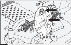
4. Confirm measurements once again. The blade tip height must be equal side to side. In the rear, the blade tips must be 1/8" to 3/8" higher than the front measurement. In the front, blade tips must be equal from side to side.
