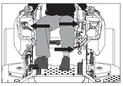
Make daily inspections to ensure that the safety system works by attempting to start the engine when one of the conditions is not met. Change the conditions and try again.
