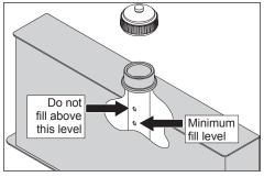
6. Reinstall the reservoir cap by hand. Do not overtighten.
