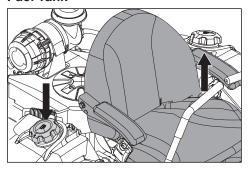
Read the safety instructions before refueling. The capacity for each tank is 20,8 liters.
