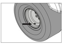
**IMPORTANT INFORMATION** DO NOT add a tire liner or foam fill material to the tires. Excessive loads created by foam filled tires will cause premature failures.
