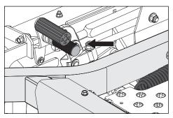
The cutting height pedals release the deck lift and set the desired deck height. Apply pressure to the lift pedal and rotate foot to also apply pressure to the release pedal, unlocking the deck lift.
