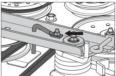
Remove the belt from around the electric clutch on the engine shaft.
