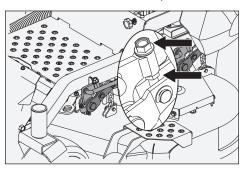
4. Confirm measurements once again. The blade tip height must be equal side-to-side. In the rear, blade tips must be 3,175 mm to 9,525 mm higher than the front measurement. In the front, blade tips must be equal from side-to-side.
