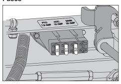
Fuses are located on the right hand side of the machine and are accessed by tilting the seat forward. Fuses are flat pin fuses type as used in automobiles. The 20 A is the primary fuse. The 7.5 A is for the mower deck coupling. The 10 A is for accessories.
