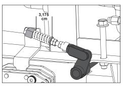
If adjustments are needed, loosen B jam nut and turn A jam nut until the correct distance is achieved. Retighten B jam nuts against A jam nuts.
