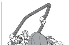
Operate the unit with the roll bar in the raised and locked position and use the seat belt. There is no rollover protection when the roll bar is down. If it is necessary to lower roll bar, do not wear the seat belt. Raise the roll bar as soon as clearance permits.
