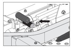
Activate the park brake, pulling the lever upwards.
