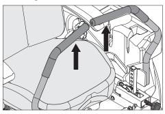
The machine's speed and direction are continuously variable using the two steering controls. The steering controls can be moved forward or backward about a neutral position. There is a neutral position, which is locked if the steering controls are moved out.
