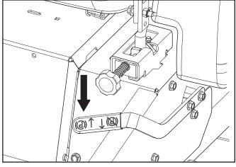
Release the parking brake to restart movement
