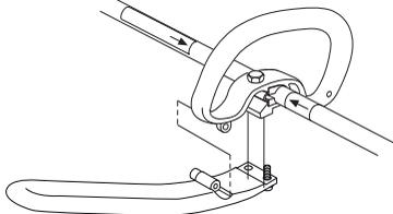
Now carry out fine adjustment to give yourself a comfortable working position. Tighten the screws.
