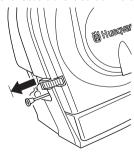
**Primer bulb:** Press the air purge repeatedly until fuel begins to fill the bulb. The bulb need not be completely filled
