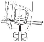
Place these on the pipe bend so that the guide on the wear ring halves aligns with the slot on the pipe bend.
