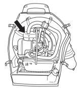
The muffler is equipped with a special spark arrestor screen. The spark arrestor screen should be cleaned once a month. This is best done with a wire brush.
