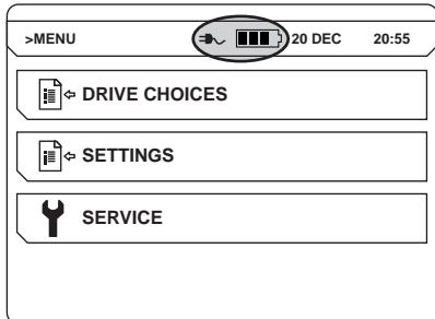
If the battery is removed while the remote control is connected to the CAN cable, the battery symbol in the remote control will be stricken through to indicate that there is no battery available.
