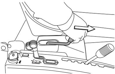
In order to ensure that the hydraulic cylinder is in the outer position, hold the lever in the forward position for a half to one second.
