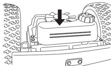
**R 422 Ts** Fill if necessary with engine oil SAE 10W/40 (class SF-CC).
