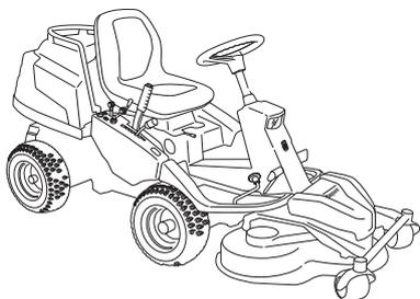
The machines are equipped with power steering and hydraulic lifts. R 422 Ts AWD also have all wheel drive.
