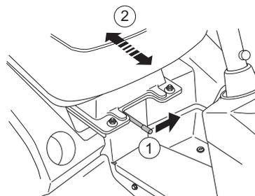
The seat springing can be adjusted by moving the rubber stops in their mountings on the underside of the seat. Place both stops in the front, middle or rear.
