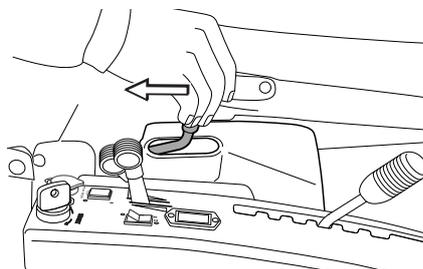
The unit can then be secured in the raised position if necessary by moving the mechanical lifting lever backwards to the lock position.
