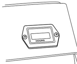
Any time when the engine is not running but the ignition is switched on is not registered. The last digit shows tenths of an hour (6 minutes).
