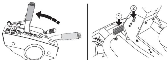
The engine can not be started if the parking brake is not pressed down.
