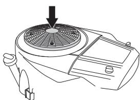
Check the air duct, located on the inside of the engine cover, ensure it is clean and does not rub against the cooling air intake.
