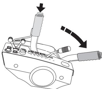
If the cutting unit does not lower completely, or if the blades do not rotate, lower the cutting unit completely using the hydraulic lifting lever. In order to ensure that the hydraulic cylinder is in the outer position, hold the lever in the forward position for a half to one second.
