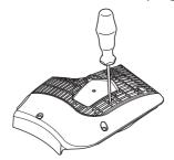
• Lubricate the recoil spring with light oil. Fit the pulley and tension the recoil spring.
