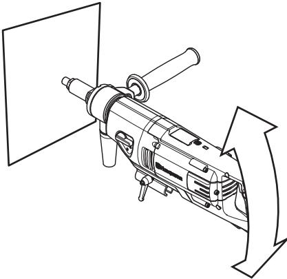
If the back of the machine is tilted downwards, the central green LED goes out and the front red LED lights up. If the back end of the machine is tilted up, the back red LED lights up.
