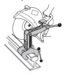
Guide the cutting blade down towards the rail and check that the cutting blade is centred in the cut. If necessary, adjust the movable bushing so that the blade ends up centred in the middle of the cut.
