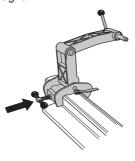
Mount the power cutter with its right side to the fixture.
