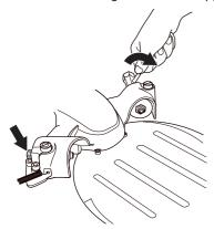
· Unscrew the adjuster screws a few turns.
