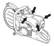
· Check the air filter and replace if necessary.
