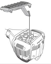
IMPORTANT! If the temperature rises above  $-5^{\circ}$ C (23°F) or 0°C (32°F) respectively the machine MUST be restored to its normal set-up. Otherwise there is a risk of overheating, which can cause severe engine damage.
