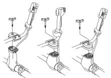
Put on the harness and hang the machine from the support hook. Now make a final adjustment so that the machine is in a comfortable working position when it hangs from the harness.
