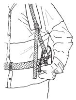
Check that the harness straps are correctly positioned. Once the harness and machine have been adjusted, check that the harness quick release works correctly.
