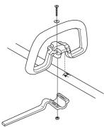
• Finely adjust the J-handle to give a comfortable working stance. Tighten the screws.
