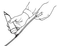
Slide the drive shaft back into the sleeve. Make sure the shaft engages correctly by turning it and pushing at the same time.
