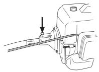
• Remove the clip that holds the throttle wire against the drive shaft.
