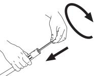
• When the shaft is correctly installed in the sleeve, the end of the shaft should project about 10 mm beyond the edge of the sleeve.
