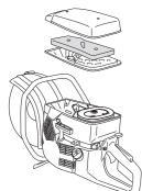
If the machine is low on power, difficult to start or runs poorly at idle speed: always check the spark plug first before taking any further action. If the spark plug is dirty, clean it and check that the electrode gap is 0.020 inch (0.5 mm). The spark plug should be replaced after about a month in operation or earlier if necessary.
