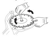
NOTICE! It is very important that the blades rotate when the nut is tightened. This is to ensure that the belt is not clamped between the integrated drive belt halves on the blades when the blades/drive belt are pulled together with the nut. Ideally this is done alternately, i.e. tighten a little, rotate a little and repeat until the blades are secured.
