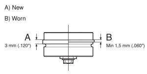
Replace the support rollers when the roller surface is flat, (or) when the groove on the roller surface has worn away.
