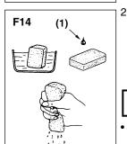
2. Use neutral detergent and warm water to clean the filter element. After cleaning, air dry the element completely and moisten with a small amount of 2 cycle motor oil.
