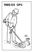
or hold the fins from the work surface during sweeping. When sweeping narrow areas such as sidewalks, the RedMax Sweeper can
