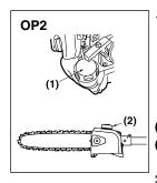
Feed fuel into the fuel tank and tighten the cap securely. (OP2)(1) (PS-EX only) Feed the chain oil into the oil tank and tighten the cap securely, too. (OP2)(2)
