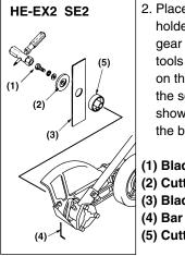
2. Place the blade between the cutter holders (A) and (B) while locking the gear shaft by putting the bar, one of the tools provided, through the key holes on the holder(A) and the gearcase. Use the socket and the screwdriver as shown in the picture below to tighten the blade mounting bolt. (SE2)
