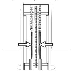
3 If necessary, the wires can be adjusted by tightening the adjuster nuts on each side of the steering collar. Do not over tighten the cables; they should only be drawn in towards the steering collar.
