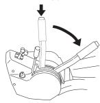
The lever can also be used to temporarily regulate the cutting height, e.g. for a small mound in the lawn.
