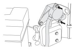
The filter can when necessary be cleaned with a brush.
