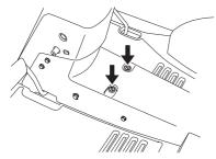
2 Check the tension of the steering wires by pushing them together (at the arrows). It should be possible to push them together so that the distance between them is half as much, without using unnecessary force.
