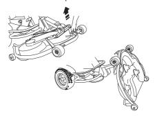
If the cylindrical bolt, which is now holding the cutting unit is removed, the cutting unit can be lifted off.
