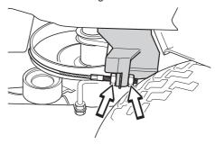
Hold the cable, for example using an adjustable wrench, so that it does not twist. If the adjustment is only made on one side, the middle position of the steering will be affected.
