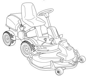
The power transmission from the engine is handled by a hydrostatic gearbox, which allows variable variation of the speed by using the pedals.
