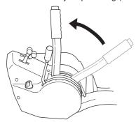
If the lock button is pressed in and the lever is moved forwards the unit will be lowered and the blades will automatically start to rotate (mowing position).
