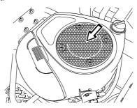
Check the air duct, located on the inside of the engine cover, ensure it is clean and does not rub against the cooling air intake.
