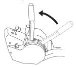
1 Pull back the throttle and turn the ignition key to the "STOP" position.
