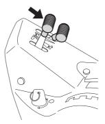
If the engine is cold move the choke lever backwards to its end position.
