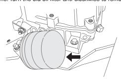
If necessary, use a filter remover.
