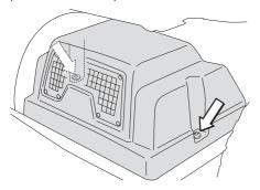
2 Check that there is oil in the transmission's oil tank. Fill if necessary with engine oil SAE 10W/40 (class SF–CC).
