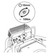
Temperature variations and vibrations can mean that the tightening torque for the screws drops. The screws should be checked when servicing to guarantee the correct torque. The tightening toque should be about 10 Nm. Never use a machine that has a faulty muffler.
