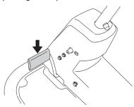
2 Carefully press down one of the pedals until the required speed is obtained. Pedal (1) is used to drive forwards, and pedal (2) to drive backwards.
