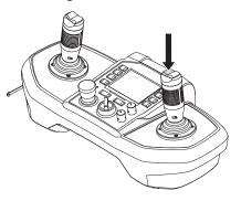
If no command is given within three seconds the operating functions are locked. To return to work mode, press the left button on the right joystick.
