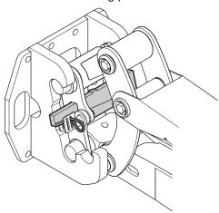
Connect the hydraulic hoses and any hoses for hammer lubrication (when fitting the hammer). The tool's pressure connection must be connected to the main valve's B-port and the return hose to the main valve's A-port.
