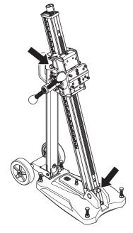
Loosen the locking screws for column tilt and set the desired drill angle. Tighten the locking screws. Use the feed lever. The column can be tilted  $0-60^\circ$ .
