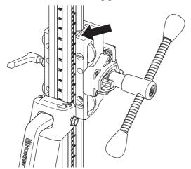
Start with the top guide roller. Use a flat screwdriver and turn clockwise to guide the roller closer to the column.
