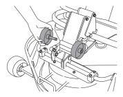
4 Fit the support wheels on either side of the rear of the cutting unit.
