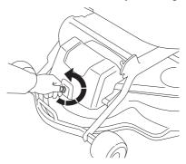
3 Loosen the spring on the drive belt's belt idler by loosening the handle.
