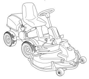
The power transmission from the engine is handled by a hydrostatic gearbox, which allows variable variation of the speed by using the pedals.
