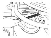
6 Place a foot on the front edge of the cutting unit near the wheel and raise the front edge of the unit to make it easier to remove the lift strut.
