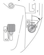
**IMPORTANT INFORMATION** Do not run the starter for more than about 5 seconds at a time. If the engine does not start, wait about 10 seconds before trying again.
