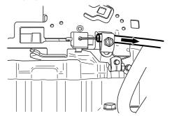
3 Pull back the throttle to the full throttle position and check that the choke is no longer actuated.
