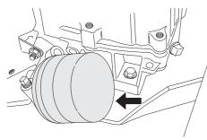
If necessary, use a filter remover.
