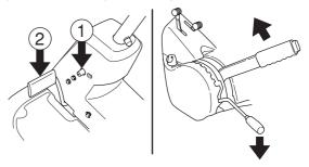
2 Remove the front hood by removing the pin.
