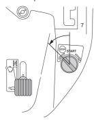
2 When the Rider is at a standstill, press down the parking brake and push in the locking button.
