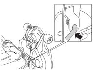
2 Replace the cutting height stay and the belt. Tension the belt with the belt adjuster.
