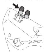
If the engine is cold move the choke lever backwards to its end position.
