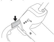
2 Carefully press down one of the pedals until the required speed is obtained. Pedal (1) is used to drive forwards, and pedal (2) to drive backwards.
