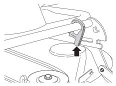
5 Lift off the drive belt and hang on the load-relieving hook.
