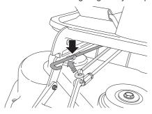
7 Grip the front edge of the unit and pull forwards until it stops.
