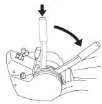
The lever can also be used to temporarily regulate the cutting height, e.g. for a small mound in the lawn.
