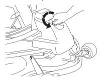
3 Remove the two support wheels from under the front hood.
