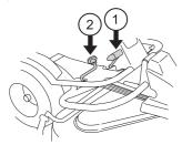
3 Select the required cutting height (1-7) with the cutting height lever.
