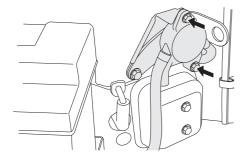
The filter can when necessary be cleaned with a brush.
