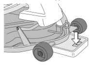
3 Adjust the unit's ground pressure by screwing in or out the adjusting screws located behind the front wheels on both sides.
