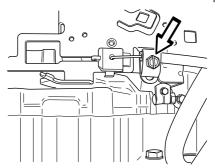
Pull the choke wire casing to the far right and tighten the clamping screw.
