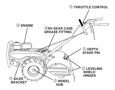
①SAE 30 OR 10W-30 MOTOR OIL ②REFER TO MAINTENANCE "ENGINE" SECTION ③EP #1 GREASE
