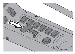
Engine speed control in idling mode
