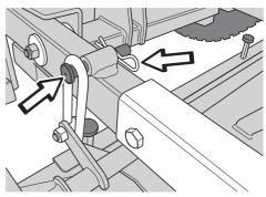
Install the pins on both sides
