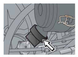
Particle trap on air filter
