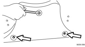
Removal of BioClip Plug
