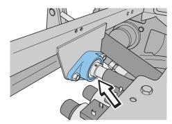
The power take-off shaft's front support bearing
