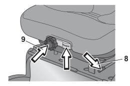
Lateral adjustment and adjusting suspension
