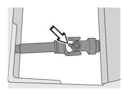
Propeller shaft's joints
