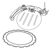
Unscrew the knob. First turn the knob a few turns until you feel a resistance. The guide roller then follows the knob out and stops when it feels a resistance.
