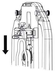
3 Lock the blade guard by pulling the handle out of the guard and then down towards the saw unit so that the latch locks the handle.
