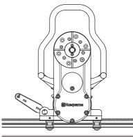
2 To secure the saw, lift the locking handle towards the saw until the handle locks.
