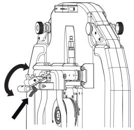
5 Connect the water hose from the out-coupling on the saw motor to the in-coupling on the blade flange hub.
