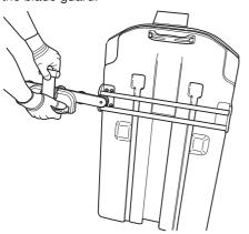
2 Make sure that the pivot arm is positioned vertically. Lift the blade guard over the blade and hang the guard in the blade guard holder on the saw. Exercise care so that the runners on the blade guard are positioned in the slots on the water block.
