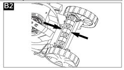
location pegs as illustrated in fig.B1 3. Clip the roller together to secure it into position.(B2)
