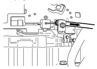
3 Pull back the throttle to the full throttle position and check that the choke is no longer actuated.
