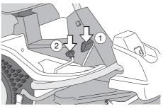
3 Select the required cutting height (1-9) with the cutting height lever.
