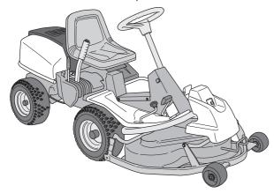
The power transmission from the engine is handled by a hydrostatic gearbox, which allows variable variation of the speed by using the pedals.
