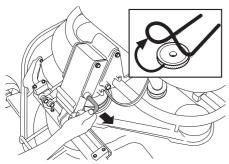
3 Pull the frame forwards and refit the pin.
