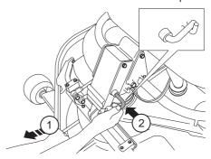
4 Grasp the front edge of the cutting unit, pull out and raise into the service position.
