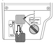
When the Rider is at a standstill, press down the parking brake and push in the locking button.
