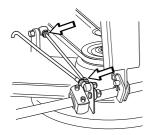
4 Screw out (extend) the stay to raise the rear edge of the
