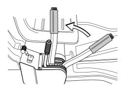
1 Pull back the throttle and turn the ignition key to the "STOP" position.
