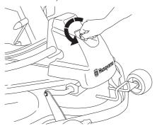
3 Remove the two support wheels from under the front hood.
