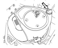
The dipstick should be completely screwed down
