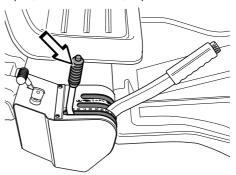
4 Press in the lock button on the lifting lever and lower the cutting unit.
