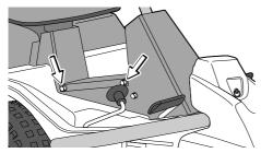
2 Check the tension of the steering wires by pushing them together (at the arrows). It should be possible to push them together so that the distance between them is half as much, without using unnecessary force.
