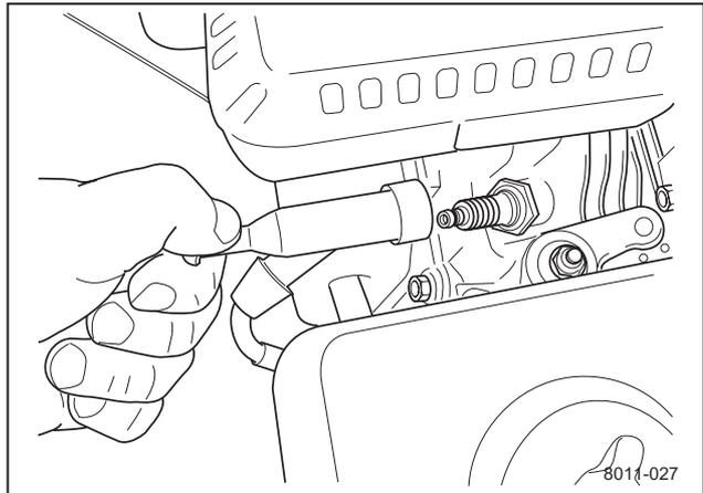
*Remove the spark plug cable*
