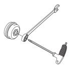
Lubricate using bearing grease inside the rollers before the new rollers are fitted.
