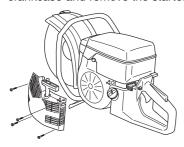
Pull out the cord approx. 30 cm and hook it into the notch in the rim of the pulley. Release the recoil spring by letting the pulley rotate slowly backwards.
