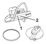
Run the drive belt over the cutting head's belt pulley (2).
